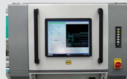
State-of-the-art Auto Optical Inspection System that zooms in on every solder joint
