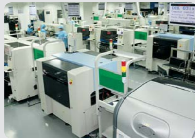
Cutting-edge Surface Mount Technology (SMT) makes fast and accurate work of loading circuit boards with miniaturized electronic components
