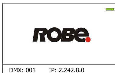
Note: The green icon at the top right corner of the screen indicates the level of the display battery charging. If the whole icon is green, the battery is fully charged while the red icon indicates exhausted battery. The battery charges during fixture operation, its charging lasts cca 6 hours.
