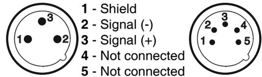
If you are using the standard DMX controllers, you can connect the DMX output of the controller directly with the DMX input of the first fixture in the DMX-chain. If you wish to connect DMX-controllers with other XLR-outputs, you need to use adapter-cables.
