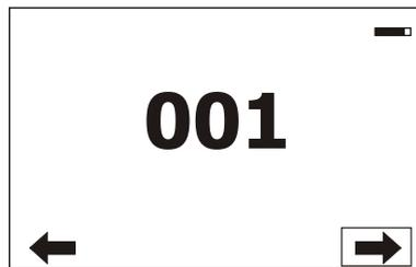
Each item (such as a Tab, menu item, text box, icon) may be selected from a screen by simply touching the item in the list or by pressing the [NEXT] or [PREV] buttons to scroll through list items. With each press, the next item is highlighted. Press [ENTER/Display On] to select the highlighted item.
