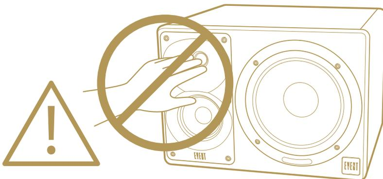
To prevent damage, do not touch the aluminium alloy tweeter dome
