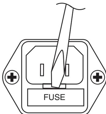
3. Remove the fuse and replace it with an equivalent-type fuse.
