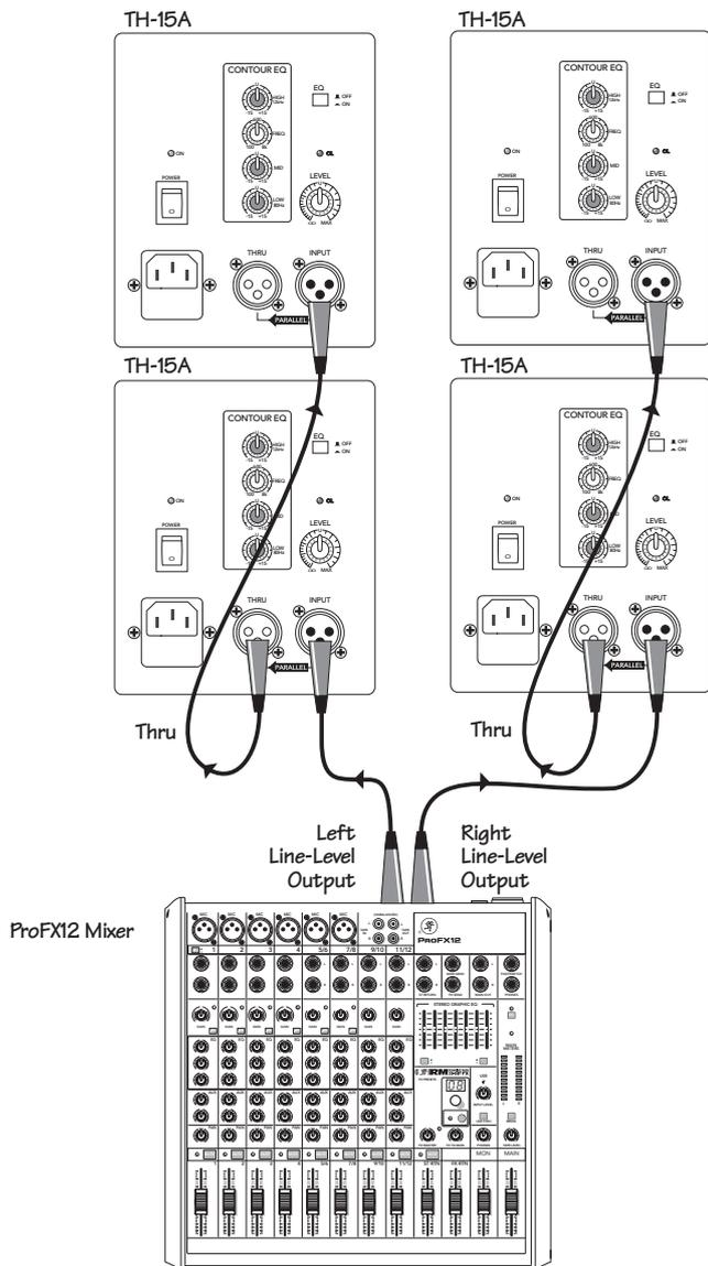
The left and right line-level outputs from a mixer feed the inputs of two Mackie TH-15A Powered Loudspeakers. Their respective THRU jacks feed the inputs of another pair of Mackie TH-15A Powered Loudspeakers.
