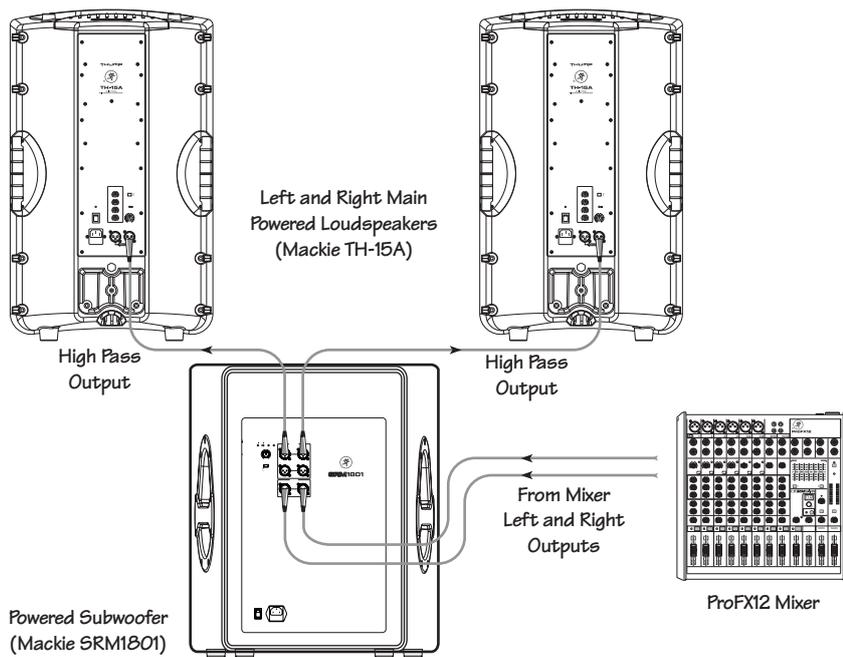
The left and right line-level outputs from a mixer feed the inputs of a powered subwoofer. The high pass line-level outputs of the subwoofer feed the inputs of the Mackie TH-15A loudspeakers.
