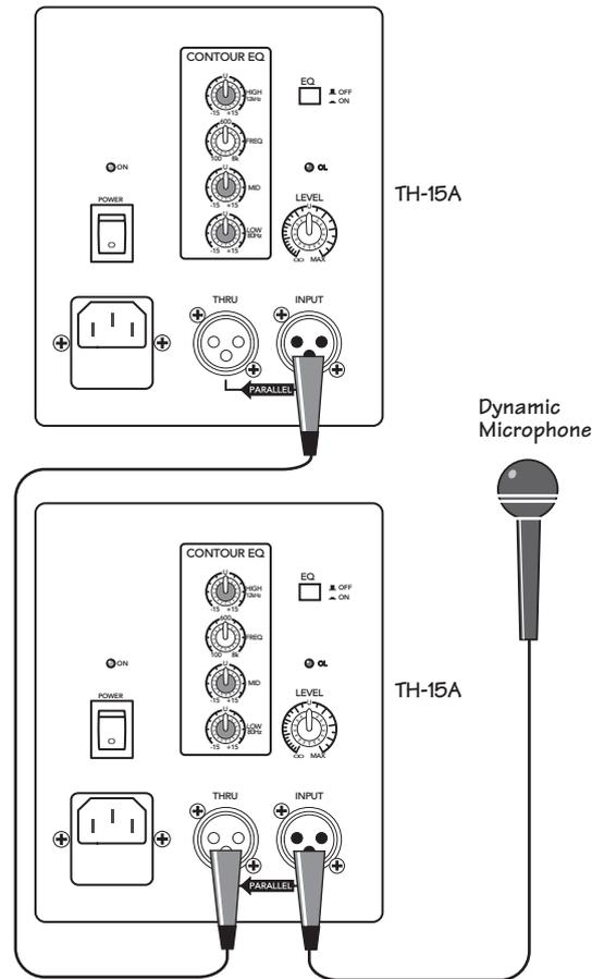
For microphone connections, you can daisy-chain up to two TH-15As using the THRU jack, as shown.
