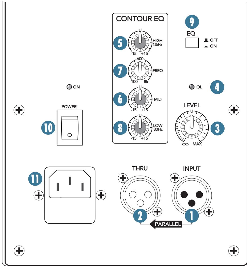
This is where you connect AC power and your signal to the loudspeaker and make adjustments to the frequency response of the speaker to match the loudspeaker's location and your room's environment.
